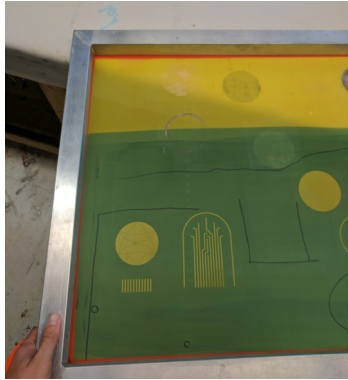
Figure 2: Silkscreen used to create printed circuit. Yellow mesh with photo emulsion.
